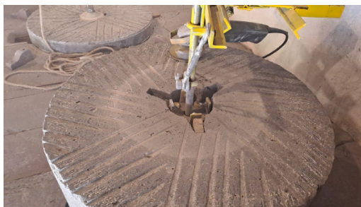
Fig 9. The swallow, ground in the bedstone with the same tool. The turnbuckle sets the angle.
