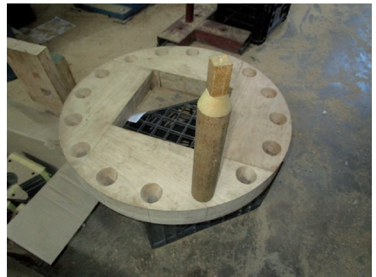
Jig to test meshing of partly finished cogs, at 10 degrees if tilt.
