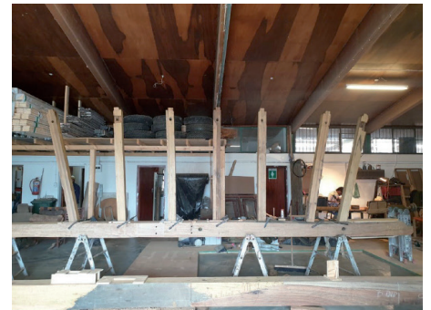
The beginnings of the tail beam, which will be beefed-up, back and underneath.
