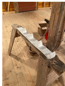
Sample meal elevator bucket pitch. Food grade belts and cups. Stainless hardware.
