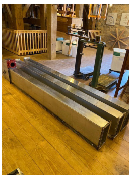
Custom stainless elevator sections for organic stones. 30' discharge height. Slide gate access on every floor level for clean out.
