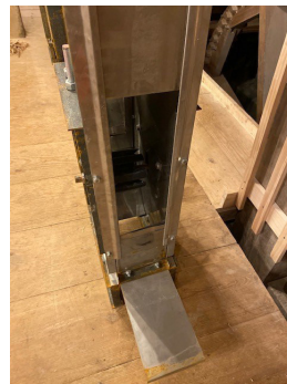
Vertical and horizontal slide gates on boots allow for easy clean out.
