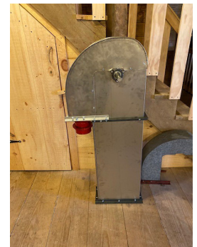
Custom food grade stainless steel elevator head. Minimum conveyance 110 bushels/hr. The head pictured is for non-organic grain and has a 24'6" discharge height.
