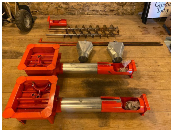
Grain sinks for unloading of 1 ton grain totes and conveying to bucket elevator. 6" augers, feed valves and slide gate controls.
