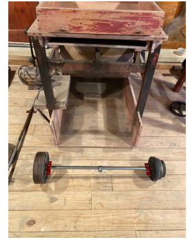
New Clipper grain cleaner shaft and bearings to accept belt drive.
