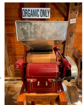
Roller Mill- 12"x6" capacity of 350lbs/hr @ 3hp. 20 corrugations per inch.
