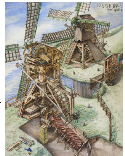
Drawing of two hollow post mills in Friesland by Anton Sipman, 1947
