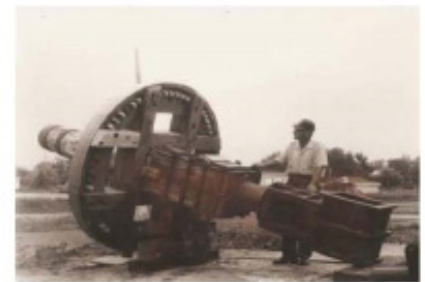
Above: Harvey Sorensen checks out the original wind shaft and brake wheel.
