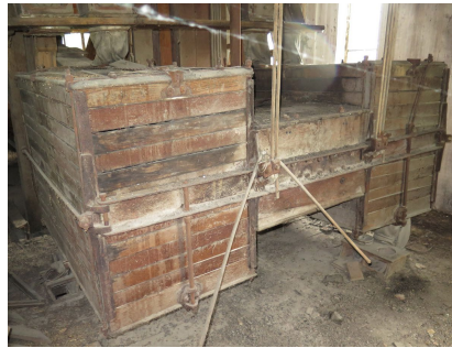
06 Plansifter suspended from bamboo canes
