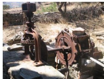
A persian wheel in Andros with a chain and metallic buckets
