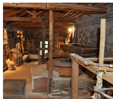
Figure 2: The internal of Morogiannis watermill. The millstone the grains silo and the flour container are visible.
