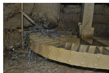
Figure 4: The water wheel (1) and the nozzle (2)
