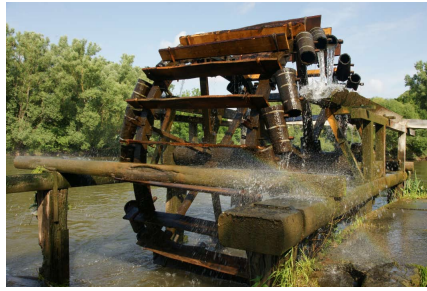
A view of a wheel with buckets on the inner and outer rim
