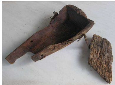
Shoe (the lower left side which sticks out is the vibrating rode for the shoe)
