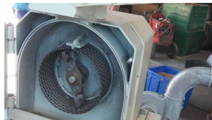
The Heger Spelt Peeler works like a hammer mill
