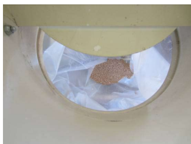
Clean grain pours off the top end of the shaking screen, down a chute and falls into a bag.
