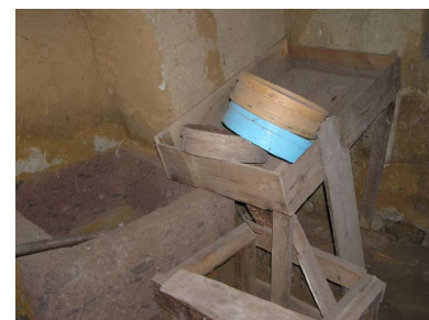
The straining box (right) and the moistening basin (left)
