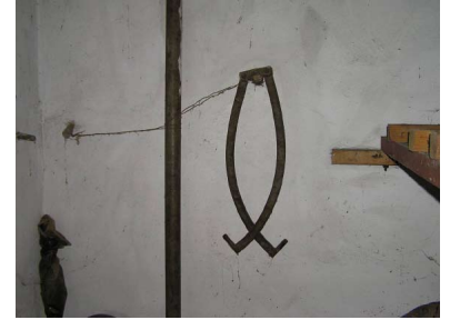
The crane for lifting the upper millstone, so it can be cleaned
