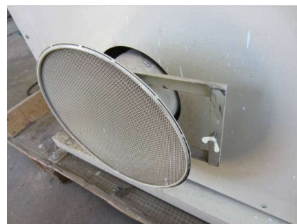
A flat slide to adjust the flow through the fan is missing.
