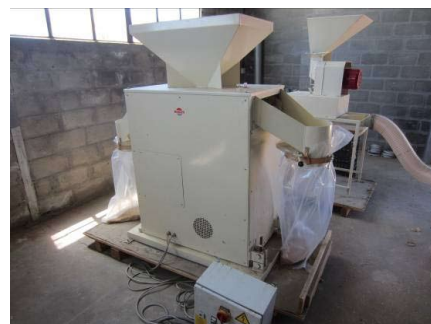
The Heger grain cleaner. Behind the electrical control box, one tilt-adjuster can be seen.
