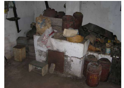
The cauldron built in the oven to boil the sesame paste
