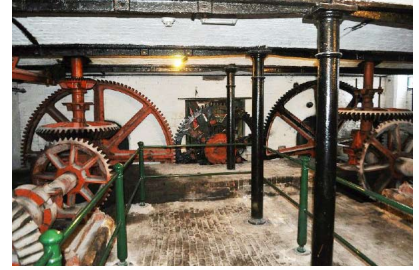
The main drive shafts and gearing
