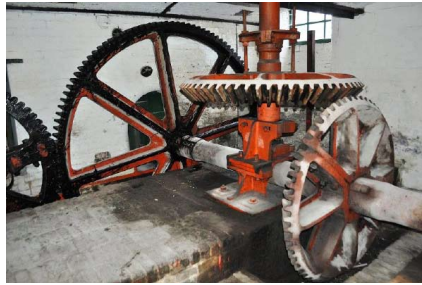
The gearing system for one grinding pan
