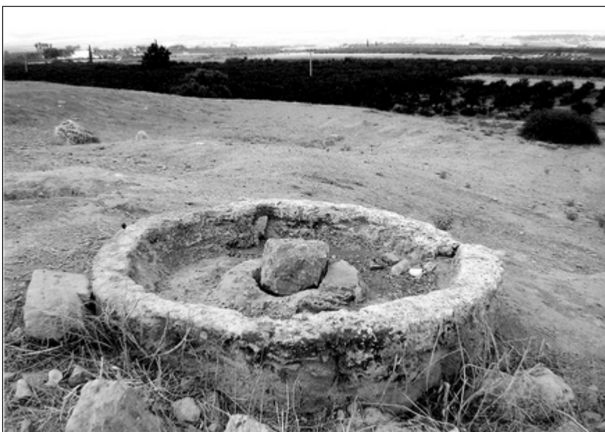
Fig. 8. The base stone at Tell aS-Sukkar showing the circular channel in which ran the edge runner.
