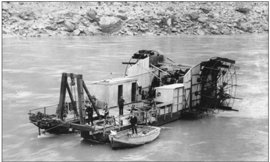
Fig. 3. Manuherikia dredge with paddle turning in a swift current and showing damaged float boards and small buckets for raising sluicing water around the inner frames of both wheels. (Reproduced by courtesy of John McCraw)
